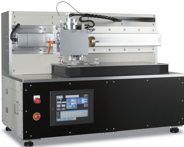
KK01 : Configurable load 1 to 200N
