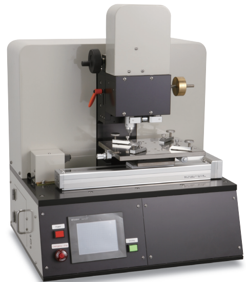
KK02 : Configurable load 1 to 50N
