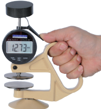
Self closing by spring force
