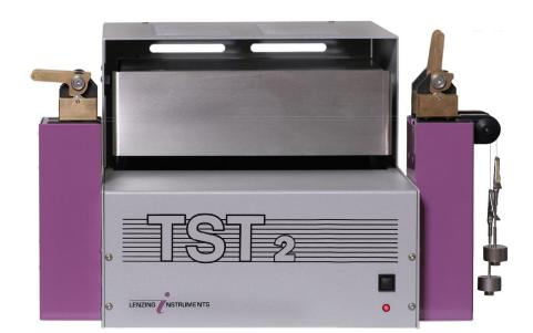
Change of length and shrinkage force at specified temperatures are two dominant quality parameters for technical and industrial as well as for textile filament yarns.
