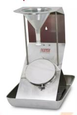
Spray Rating Tester, to determine the surface wetting resistance of fabrics, which may or may not have been given a water-resistant or water-repellent finish. Spray Rating Tester complies with AATCC 22, ISO 4920, EN24920, etc. Our Spray Tester is your best choice when you do spray test.
